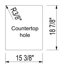
**NOTES:** Refer to installation instructions supplied with kitchen sink for undermount, or drop-in installations. Templates and installation kits provided with the sink.
